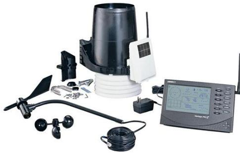
coverage exists at your site you will need to determine mounting options for your weather station. The Davis Vantage Pro II weather sensors need to be mounted within 300 yards of your console for proper reception (120 yards through walls). The instruction manual that comes with your weather station will have instructions for testing reception between your weather sensors and your console.
