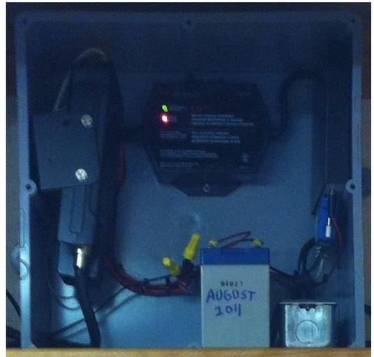
The picture on the left shows an installed project box in Buttonwillow, CA. Since the antenna cable was fished in the wall to the attic it is not visible in the picture. The box was centered and screwed directly to a wall stud through the back of the enclosure. The picture on the right shows a completed project box with the cover off.
